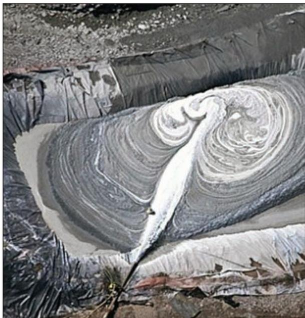
A toxic slurry pond, i.e., a pit that catches contaminated water from "fracking." Fracking is the process where water, sand and chemicals are injected into the earth at extremely high pressure to release natural gas.
