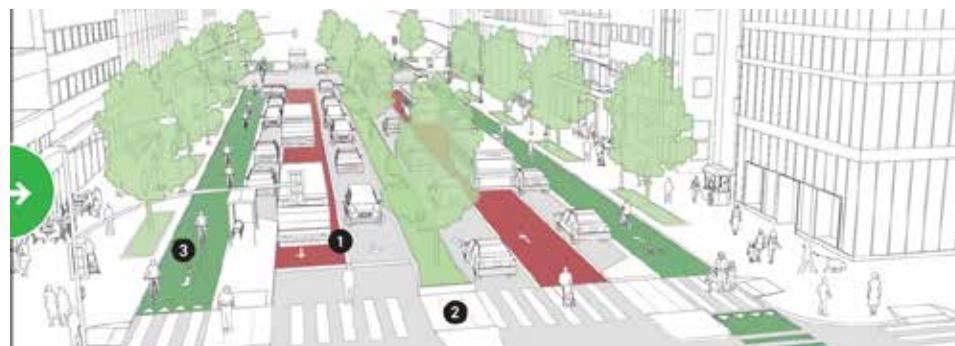
Figure 54: To reach their full potential as high transit-ridership mixed-use corridors, some streets may require major redesigns that significantly improve the pedestrian experience, reduce car capacity, and protect transit from congestion. (Above example from NACTO Global Street Design Guide, 2017.)
