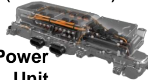
PCU-Power Control Unit (motor controller)
