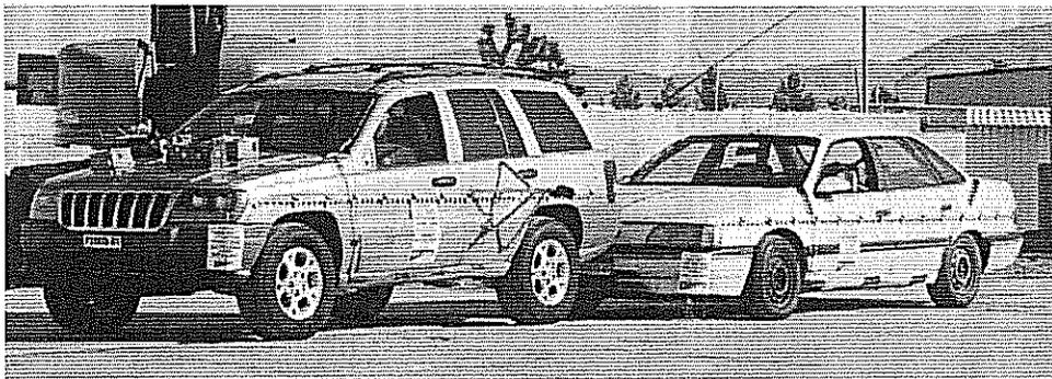
Figure 4. Test setup at Karco for offset 50 mph rear impact test.
