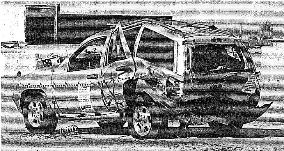
Figure 6. 1999 Jeep Grand Cherokee after 40 mph rear impact by a Taurus at Karco.
