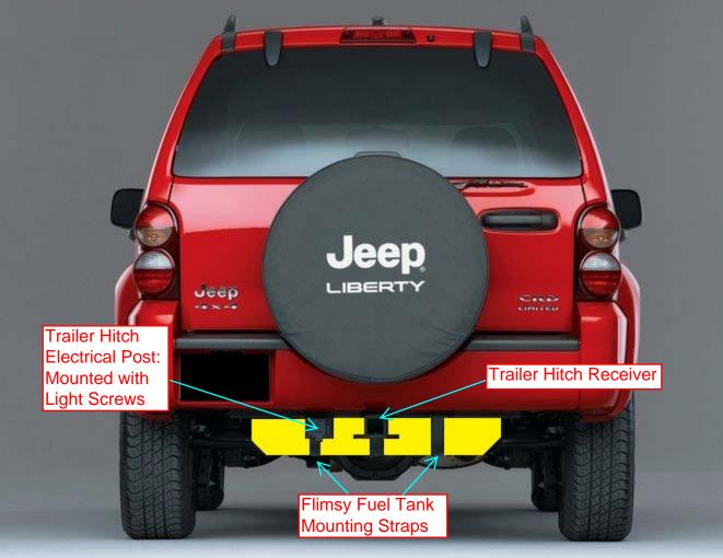
Trailer Hitch Electrical Post : Provides Electrical Spark **Ignition Source** During 'Brakes on' Collision or During 'Lights on' Normal Nighttime Running
