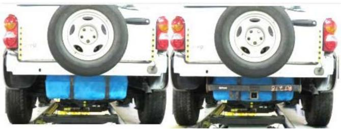
Shown in Yellow: Plastic Fuel Tank Surface that Remains Vulnerable to DIRECT Collision AFTER So-Called "Remedy"
