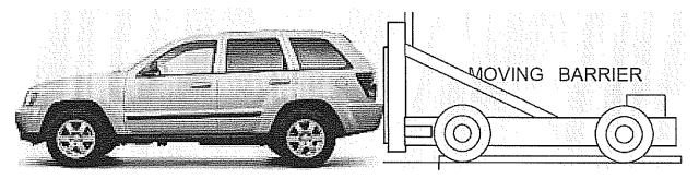
Figure 3. Diagram of FMVSS 301 (old) moving barrier impact test that was used by Chrysler to certify compliance with FMVSS 301 of its 1996 model vehicles.
