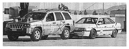
Figure 4. Test setup at Karco for offset 50 mph rear impact test.
